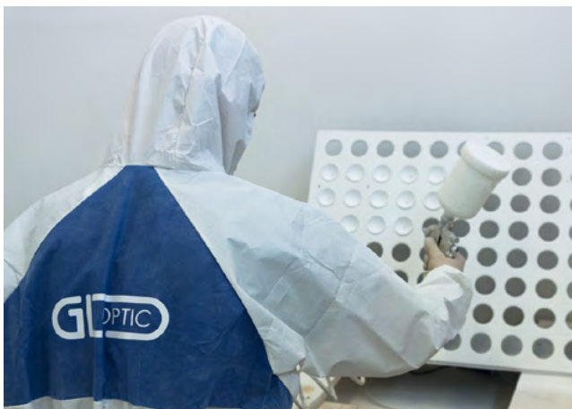
Fig. 6. Painting of integrating spheres with barium sulphate.
