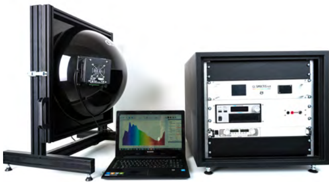
Fig. 2. Example of a complete measuring system consisting of a 50 cm diameter integrating sphere, with a Peltier module, a computer with analysis and reporting software and a spectrometer, power supply and programmable temperature controller (placed in a rack cabinet).
